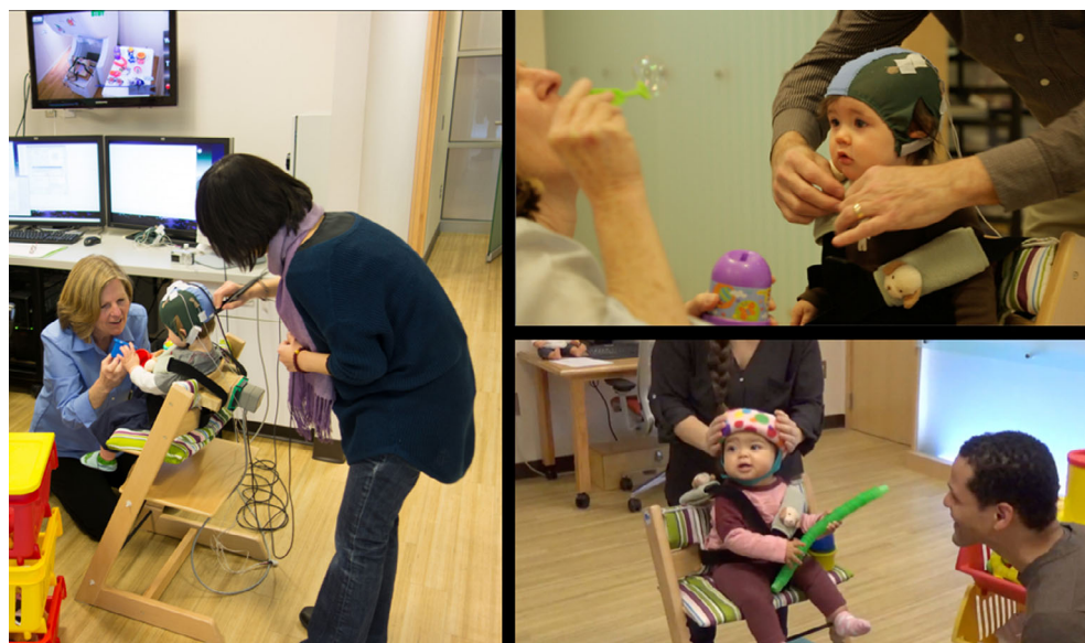
FIGURE 1 Digitization setup for use with the Polhemus device. Left panel: A toy-waver is engaging with an infant as a researcher digitizes the anatomical landmarks, head position indicator (HPI) coil locations, and additional head points. Top right panel: An infant wears a soft cap equipped with the HPI coils. Bottom right panel: A researcher places the foam halo on the infant's head before the infant is positioned under the MEG helmet
