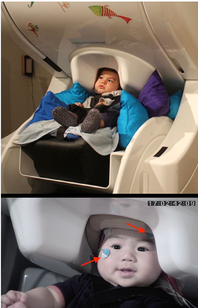
FIGURE 3 Top panel: An infant seated under the MEG dewar in the infant car seat during data collection. Bottom panel: An infant seated in the MEG system showing the placement of the two EOG electrodes (red arrow)
