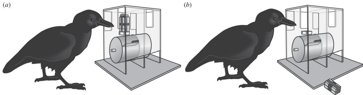
**Figure 1.** Diagram of the experimental apparatus. If the block is inserted into the hole on the upper left side of the apparatus or pushed from the ledge underneath this hole, then it falls onto the platform. This causes the platform to revolve and dispense either meat (crow experiment) or a marble (child experiment). Inserting the block into the five other holes in the apparatus (two on the back, three on the front) does not cause the platform to revolve.
